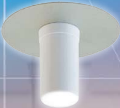
WLAN-2W (WHITE) WLAN-2B (BLACK) 2.4 GHz 3dBi INDOOR (CEILING MOUNT) OMNI WLAN ANTENNA, LONG TYPE N-FEMALE CONNECTOR, 2.5" LONG
